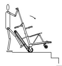
Grip the rear lifting handles push STAIRCLIMBER to next location.
