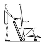
Deploy STAIRCLIMBER as shown, be sure the battery is switched on, adjust the telescopic gripping frame to suitable height.
